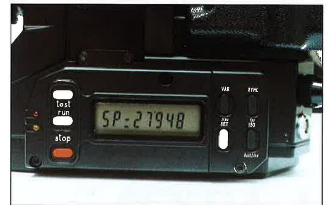
A full-function LCD display not only monitors all camera operations, but provides off-speed, misload and low battery warnings. It incorporates a mini-jog for quick setting of camera and display functions.
